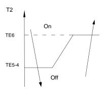
When the evaporator coil temp.T2 keeps lower than TE5-4 for 8 minutes, the compressor and outdoor fan will shut off. When T2 is higher than TE6, the compressor and outdoor fan will restart up.
