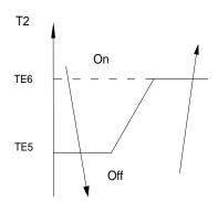
When.T2≤TE5 for Time0, the compressor and outdoor fan will shut off. When T2>TE6, the compressor and outdoor fan will restart up.
