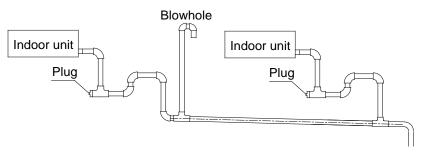
6.2.9 The end of drainage pipe shall not contact with ground directly.
