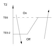
When the evaporator coil temp.T2 keeps lower than TE5-2 for 20 minutes, the compressor and outdoor fan will shut off. When T2 is higher than TE6, the compressor and outdoor fan will restart up.
