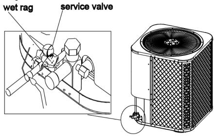
Valve can be opened by removing the plunger cap and fully inserting a hex wrench into the stem and backing out counter-clockwise until valve stem just touches the chamfered retaining wall.
