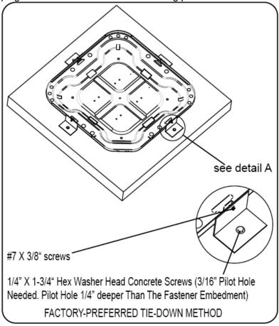
IMPORTANT: Do not use screws longer than indicated 1/4" \* 2/3" and make sure that the brace is attached on center of base ban where indicated in Fig.7. Damage will occur to system.
