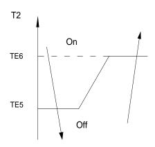
When the evaporator coil temp.T2 keeps lower than TE5 for 30 minutes, the compressor and outdoor fan will shut off. When T2 is higher than TE6, the compressor and outdoor fan will restart up.
